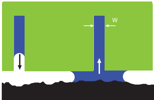
Figure 6. During separation of the toe pad from the substrate, liquid will flow back into the channels or grooves when the separation between the solid walls is larger than the width of the channels, i.e., h > W . The fluid flow direction is indicated by the vertical arrows.
